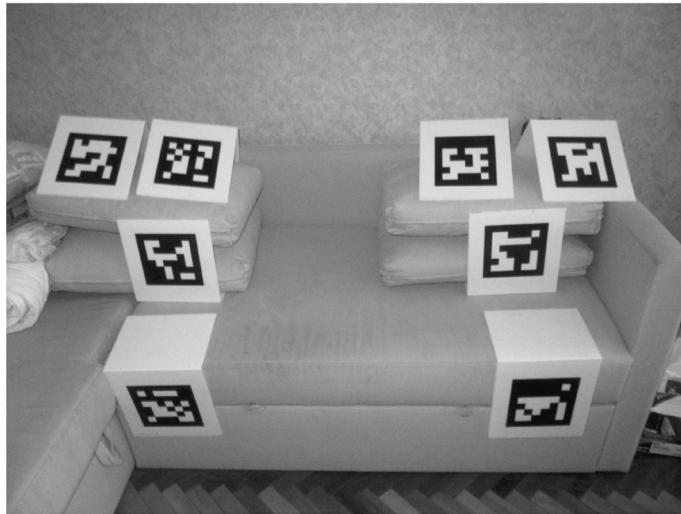
Fig. 8. A base of markers used to tie camera and object location.
